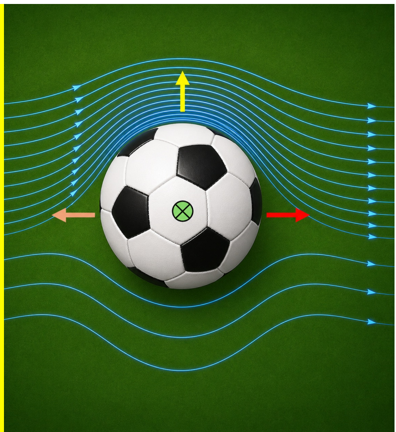
Figure 2) Simplified airflow and force diagram for a spinning soccer ball
