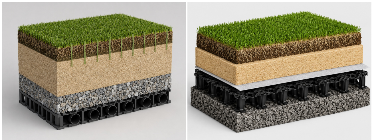
Figure 1) Educational schematics of two natural-turf stadium pitch profiles
